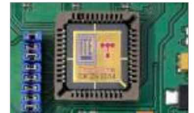
Multi-channel readout IC for FET-based THz detectors (AMS 350nm)
