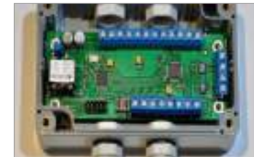
Multi-sensor node – part of the sensor network for T and RH measurements in building
