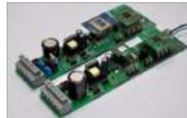
Smart luminaire controller and ZigBee - Bluetooth bridge
