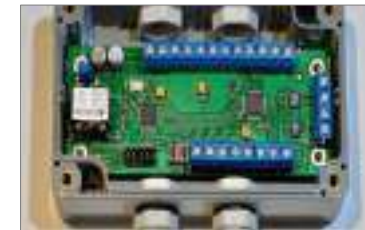
Multi-sensor node – part of the sensor network for T and RH measurements in building
